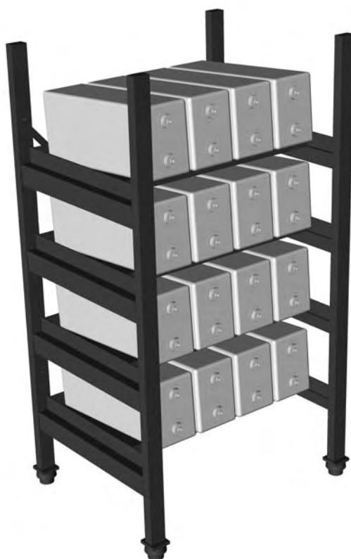
Length of the stand is determined by the combination of 5 different longitudinal beams (Length 600 mm, 750, 900, 1200 and 1500 mm) in relation with the total length of cells.
